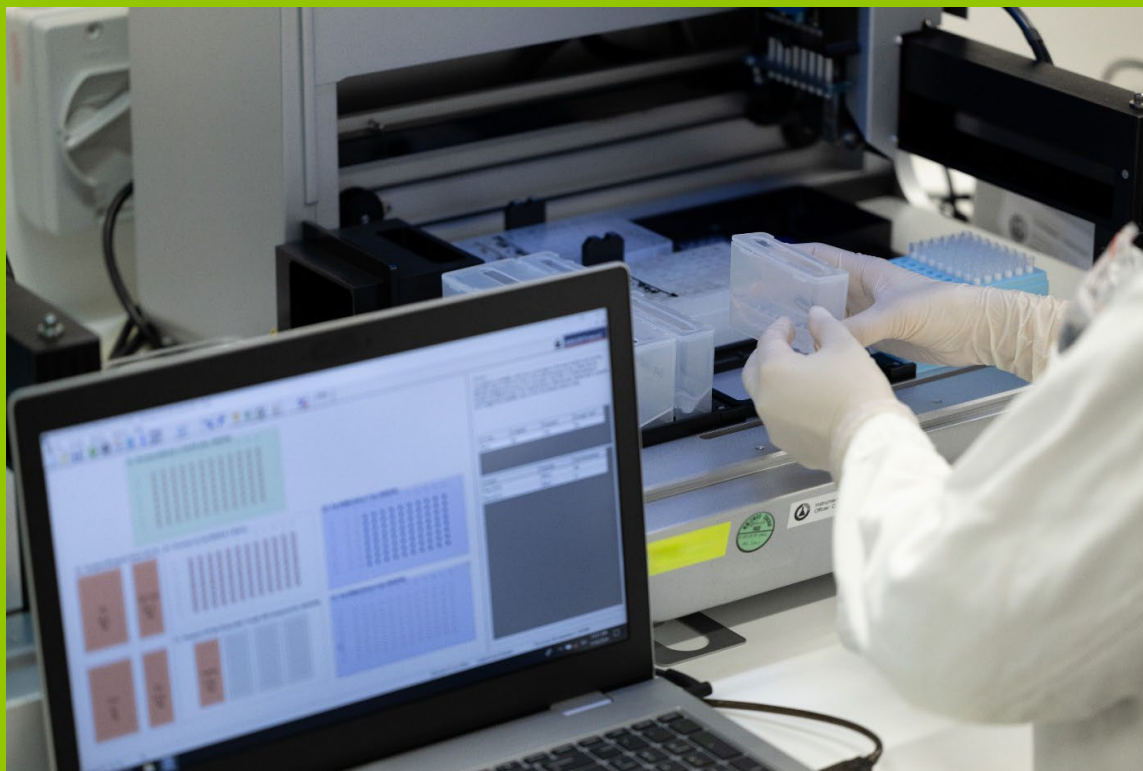
Performing DNA extraction using a robotic workstation
