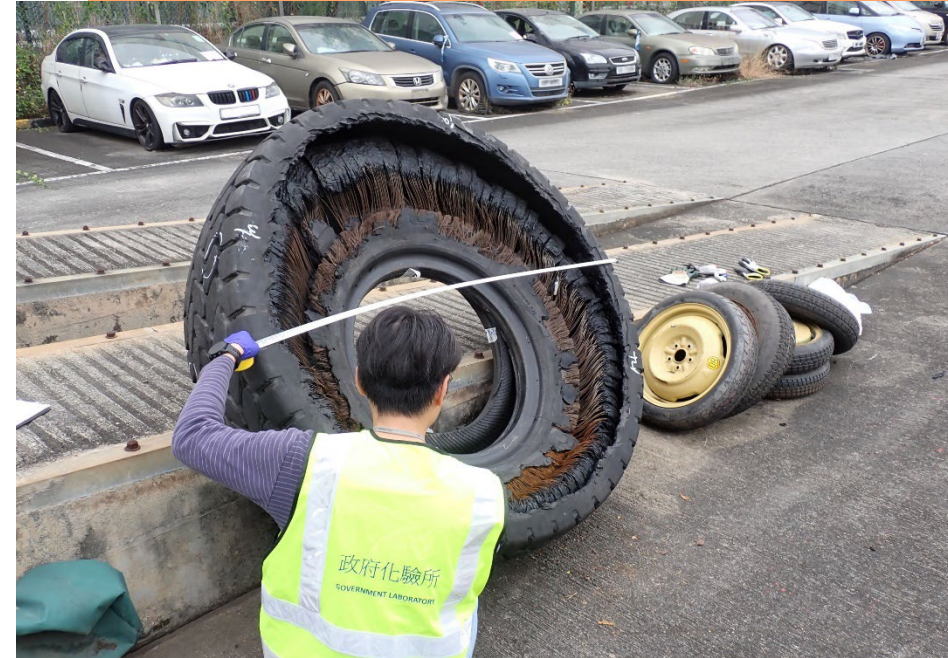
Examination of a detached tyre at vehicle detention pond
