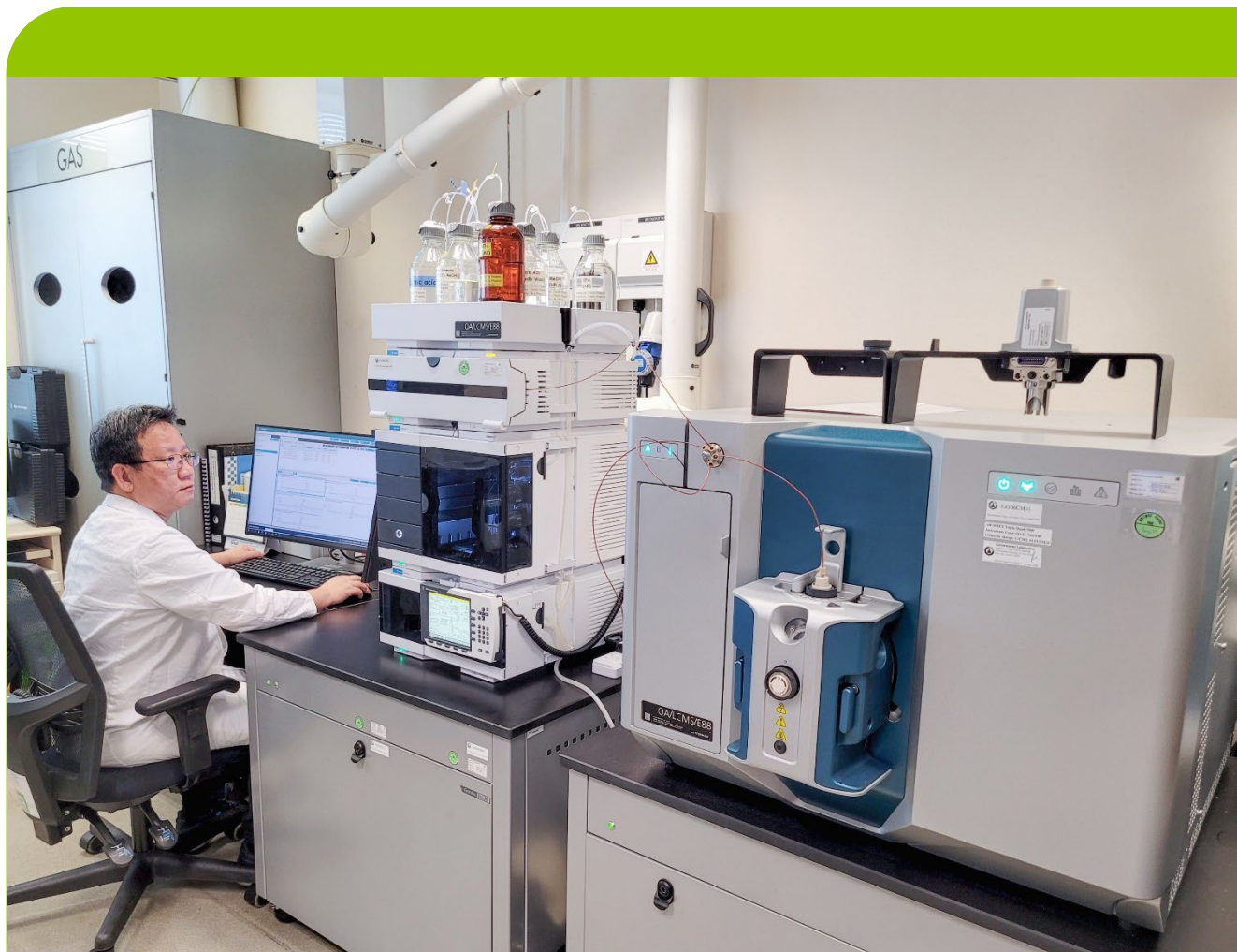
Sample analysis using liquid chromatography–triple quadrupole mass spectrometry
