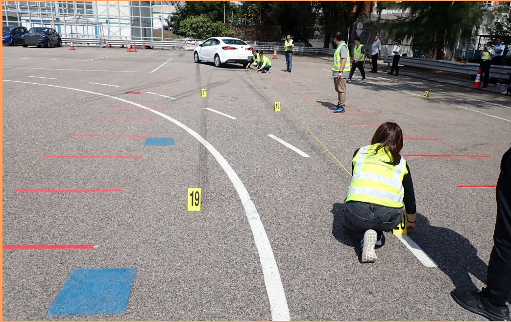
Skid mark measurement during traffic accident reconstruction
