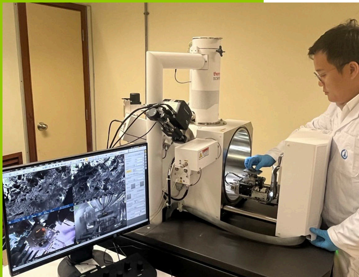
Analysis of foreign substances in a food complaint sample by scanning electron microscopy
