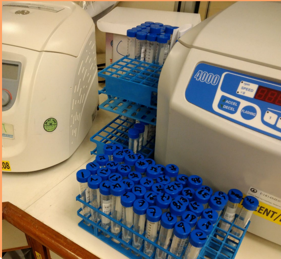
Hair sample preparation using high speed centrifuge
