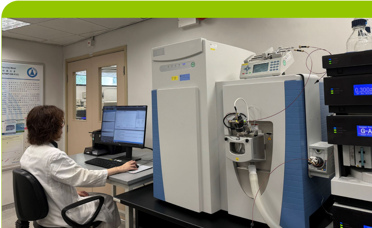
Ultra performance liquid chromatograph with quadrupole orbitrap mass spectrometer for the analysis of pesticide residues in food
