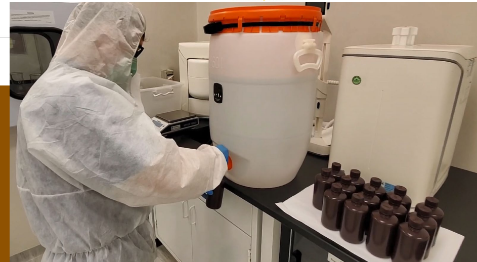
Preparation of samples in cleanroom for the supplementary comparison, SIM.QM-S12 "Trace elements in natural water", co-organised by the Government Laboratory, National Research Council of Canada (NRC) and National Measurement Institute, Australia (NMIA)
