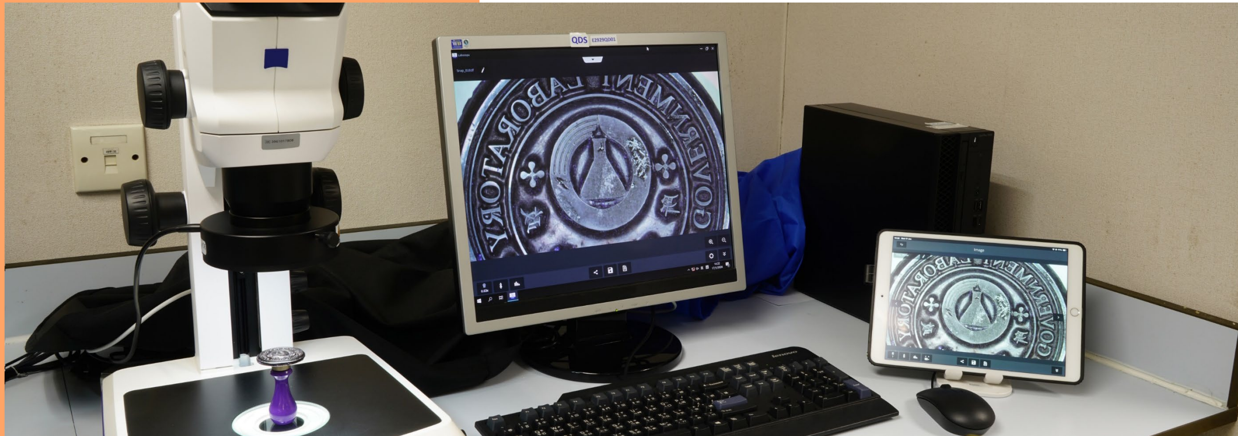
Stereo microscope for examination of exhibits (can support simultaneous viewing from multiple devices)
