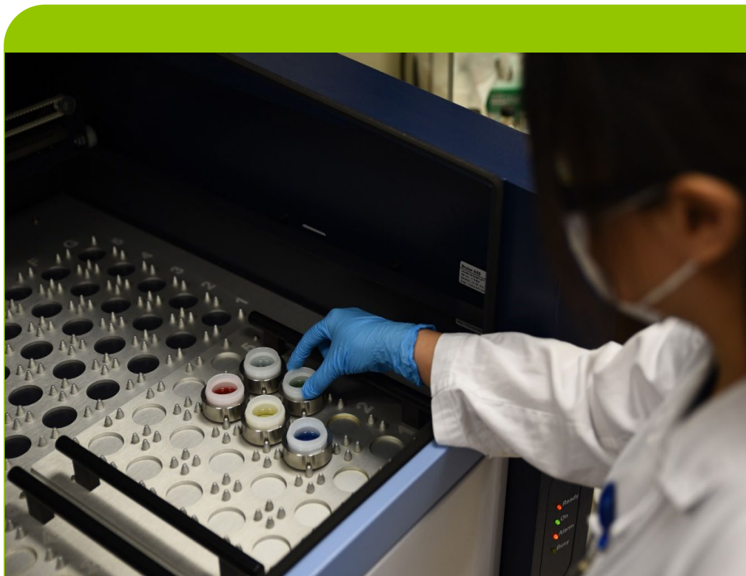
Analysis of sulphur content in fuel oil samples using wavelength dispersive X-ray fluorescence spectrometry
